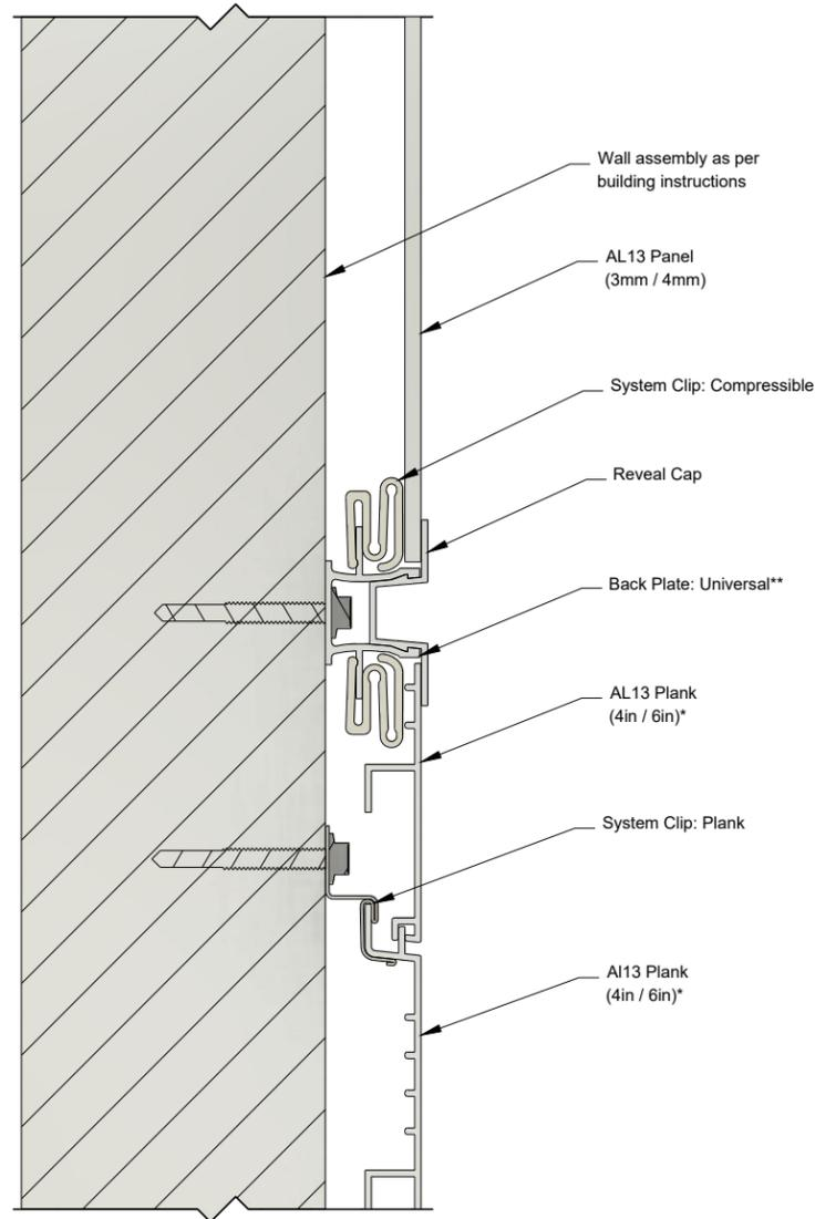
\*Plank wall termination with a ripped plank. See AL13 Panel Installation Guide for more information.
