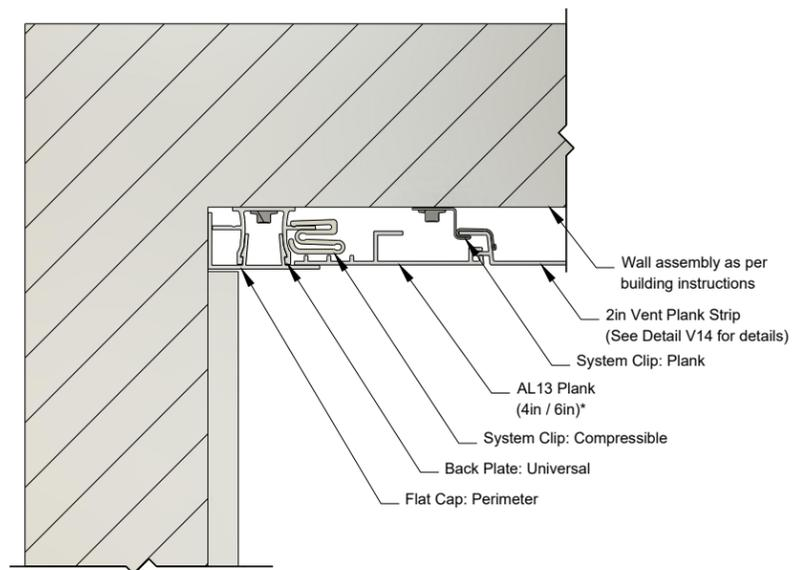
\*Plank wall termination with a ripped plank. See AL13 Panel Installation Guide for more information.
