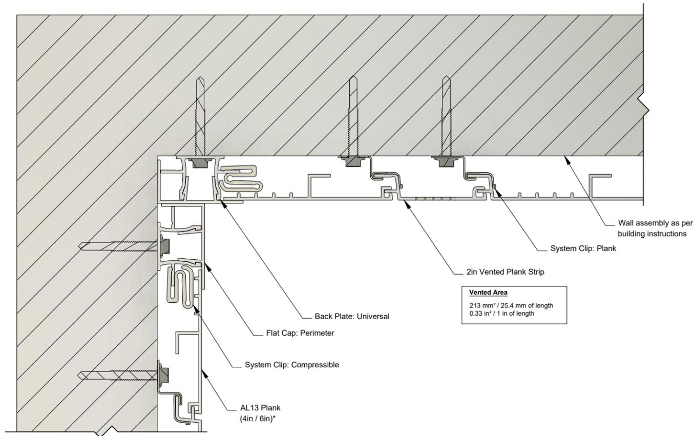
\*Plank wall termination with a ripped plank. See AL13 Panel Installation Guide for more information.
