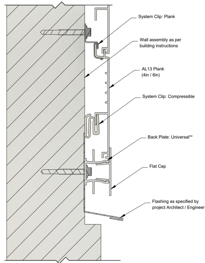
\*Plank wall termination with a ripped plank. See AL13 Panel Installation Guide for more information.
