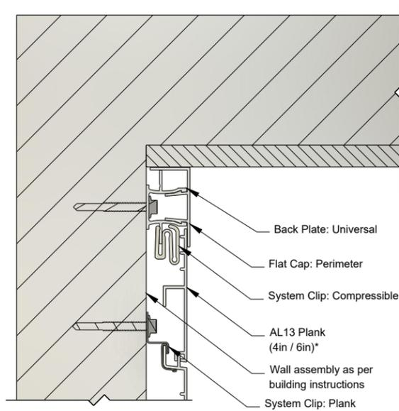
\*Plank wall termination with a ripped plank. See AL13 Panel Installation Guide for more information.
