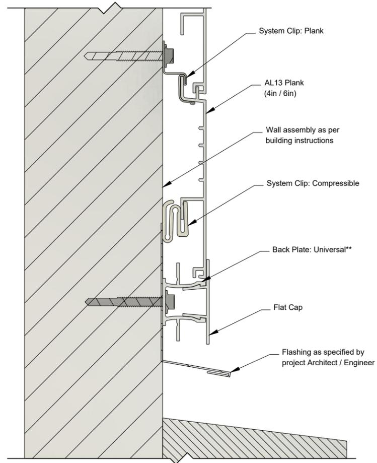
\*Plank wall termination with a ripped plank. See AL13 Panel Installation Guide for more information.
