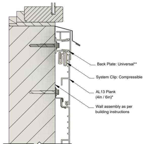
\*Plank wall termination with a ripped plank. See AL13 Panel Installation Guide for more information.
