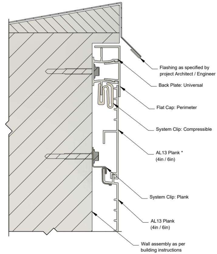
\*Plank wall termination with a ripped plank. See AL13 Panel Installation Guide for more information.
