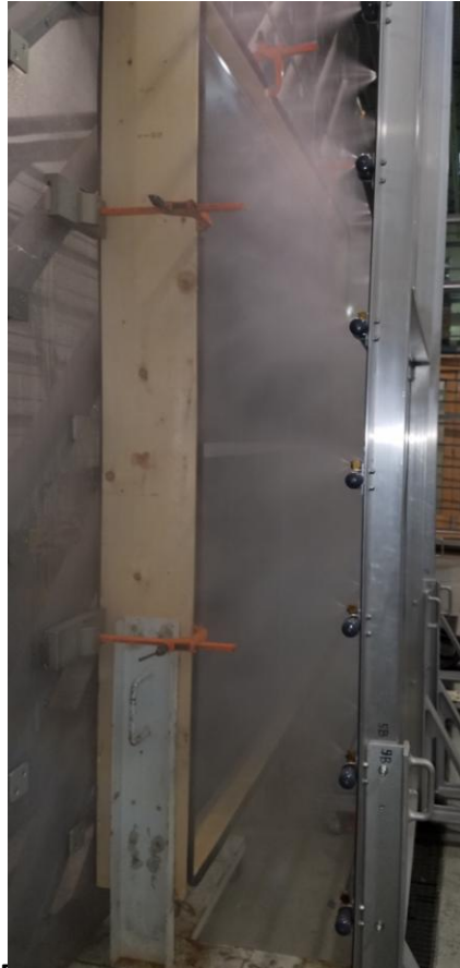
Water Penetration Resistance – Static, Test setup
